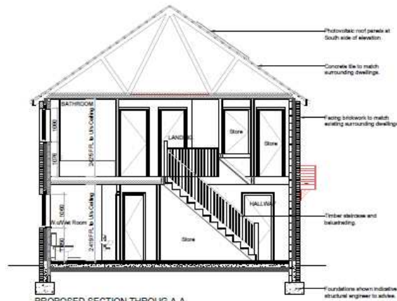
PROPOSED SECTION THROUGH A-A Scale 1:50
